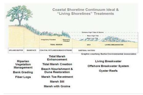
Shorelines are often stabilized with hardened structures, such as bulkheads, revetment, and concrete seawalls. Ironically, these structures often increase the rate of coastal erosion, remove the ability of the shoreline to carry out natural processes, and provide little habitat for estuarine species. Living shorelines use plants, sand, and limited use of rock to provide shoreline protection and maintain valuable habitat.
